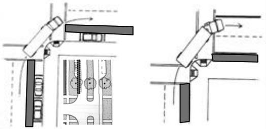
**Figure 8-6.** Adding bike and parking lanes increases the potential turning radius for oversized vehicles, while maintaining the benefits of smaller turning radii for pedestrians.
